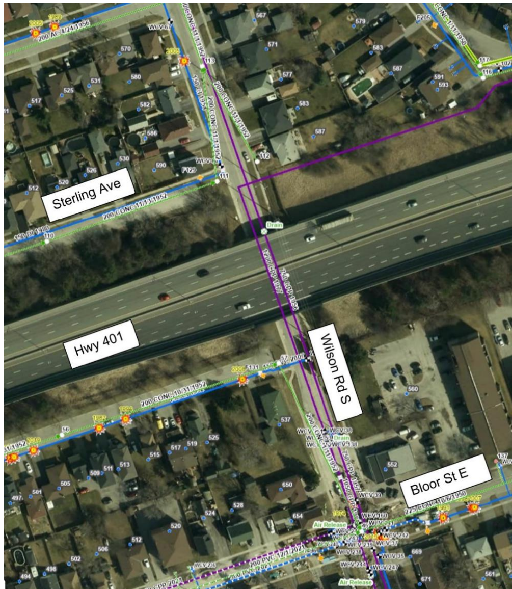
Figure 6: Existing Municipal Servicing Infrastructure along Wilson Road
